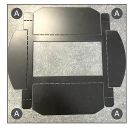
Fold **DOWN** tab corners indicated on drawing "A" to approx 90 degrees.
