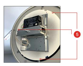
Using a PZ2 pozidrive slacken 3 x gear tray retaining screws and slide clips to the side allowing for removal of gear tray.
