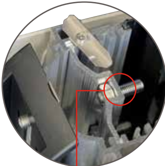
STEP 2 Move clamp to desired size
