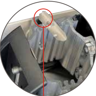
STEP 1 Twist open the locking plate
