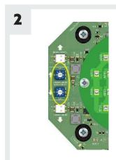
Identify the control board in the base of the beacon gallery and locate the array adjustment controls. There are two controls offering 8 levels of adjustment to the front and back projection. Note the arrows indicate which side of the beacon will be adjusted by each control.
