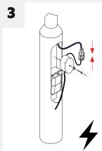
Move to the base compartment of the host post and fix the beacon transformer onto the column board using the four screw provided.
