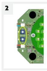
Identify the control board in the base of the beacon gallery and locate the array adjustment controls. There are two controls, each offering 8 levels of adjustment to the front and back projection. Note the white arrows printed on the board indicate which side of the beacon will be adjusted by each control each control
