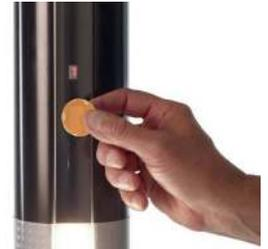
Hold the supplied magnetic wand on the marked area within the first black band. A red dot will illuminate on the display to show that the system is active. After around 10 seconds the display will illuminate to show the current lighting level. Swiping the magnet across the area will advance the lighting level making the post brighter.
