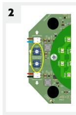
Identify the control board in the base of the beacon gallery and locate the array adjustment controls. There are two controls, each offering 8 levels of adjustment to the front and back projection. Note the white arrows printed on the board indicate which side of the beacon will be adjusted by each control.
